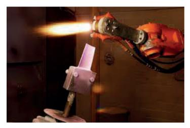
Plasma Spray technology is used to deposit abradable coatings typically used for seal closing areas improving overall turbine efficiency and performance.
